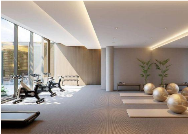
B Step Ceiling Detail + Linear Accent Lighting
